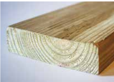
Figure 4. Some decking might initially look better with the bark side down, but eventually water can get under the grain and lift it, causing the board to peel.
