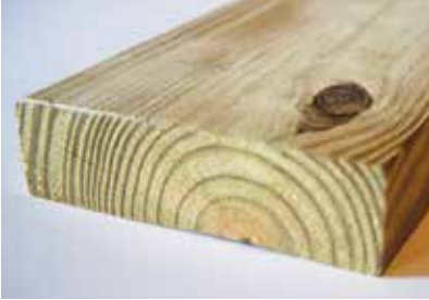
Figure 3. Even though the bark side of this decking has a knot, it should still be installed facing toward the weather.
